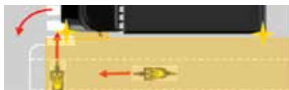
Smart BSIS and Smart LCS detecting VRU and vehicles on the Left Side
